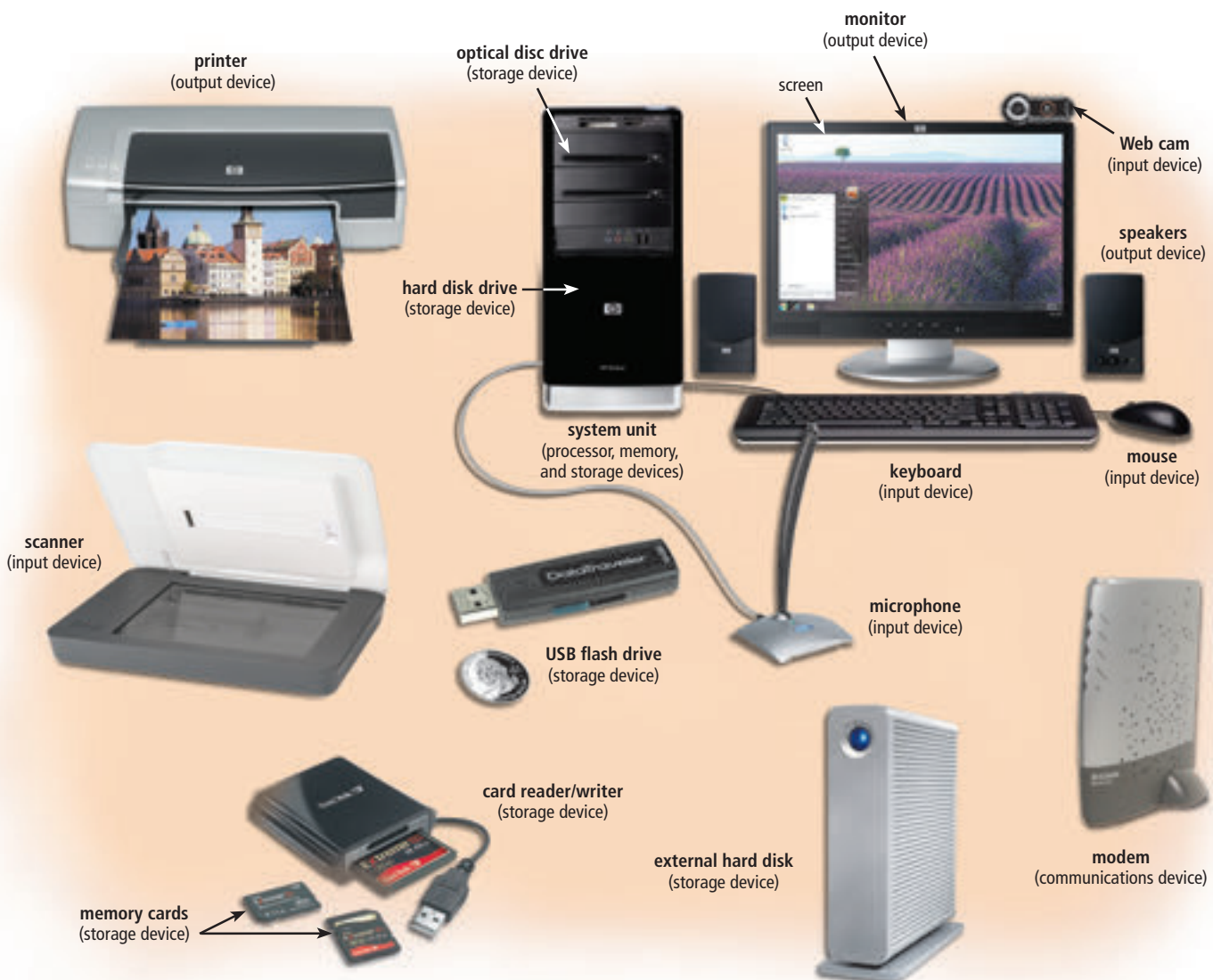
Figure 1 Common computer hardware components include the keyboard, mouse, microphone, scanner, Web cam, printer, monitor, speakers, system unit, hard disk drive, external hard disk, optical disc drive(s), USB flash drive, card reader/writer, memory cards, and modem.
