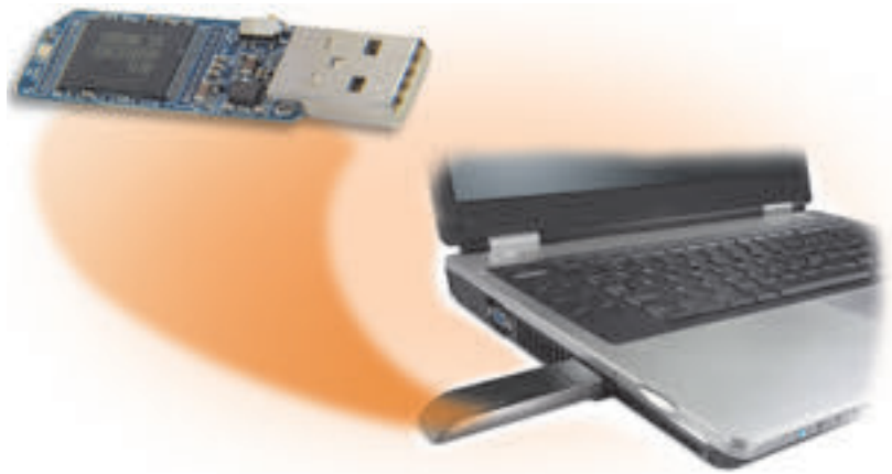
Figure 24 A close-up of the flash memory and circuitry inside a USB flash drive.
