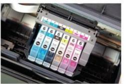
▲ Figure 1.64 Cartridges used in an inkjet printer
