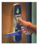
Figure 1.51 A fingerprint scanner detects unique patterns in your fingerprints
