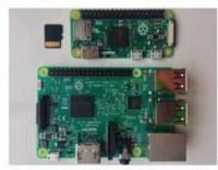
Figure 1.6 The Raspberry Pi Zero (top) and its microSD card (top left)
