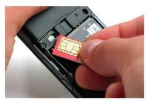
▲ Figure 1.7 The SIM card from a mobile phone
