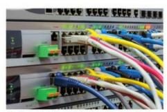
Figure 5.7 Cat5e cable is used to connect devices through their NICs
